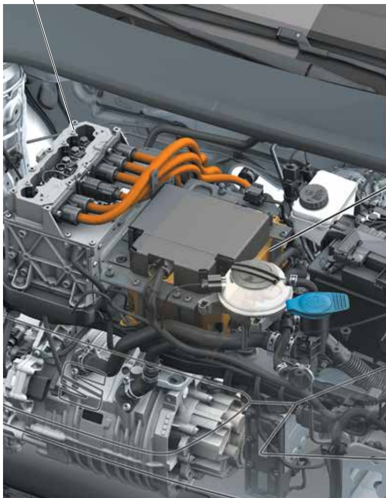
Power and control electronics for electric drive JX1
