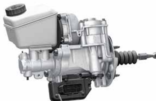
Brake servo control unit J539
