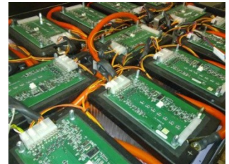
Figure 2 Battery modules with battery management boards integrated
