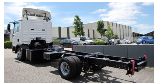
Figure 3 AGV MAN truck - battery box visible behind front wheel
